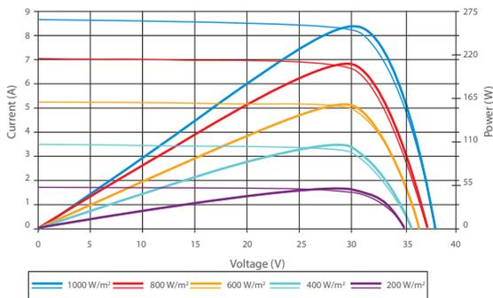
Excellent performance under weak light conditions: at an irradiance intensity of 200 W/m<sup>2</sup> (AM 1.5, 25 °C), 95.5% or higher of the STC efficiency (1000 W/m<sup>2</sup>) is achieved
