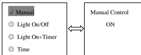
the default load output can be set ON/OFF in this interface.
