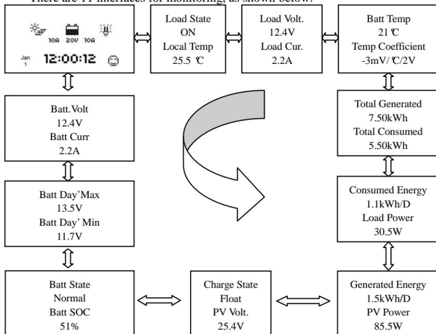
Press **OK** to enter the monitoring interface when the inverse cursor point to **monitor** item.
