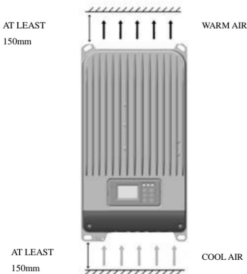
Figure3-1 Required mounting clearance for air
