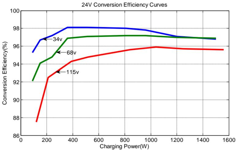
3. Solar MPPT Voltage(68V,115V) / System Voltage(36V)
