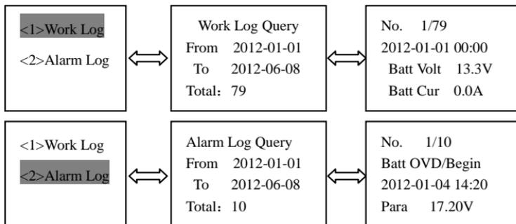
Press **OK** to enter the monitoring interface when the inverse cursor point to **monitor** item. Press **ESC** button to exit. Work Log and Alarm Log could be browsed in this interface, the operation is as follows:
