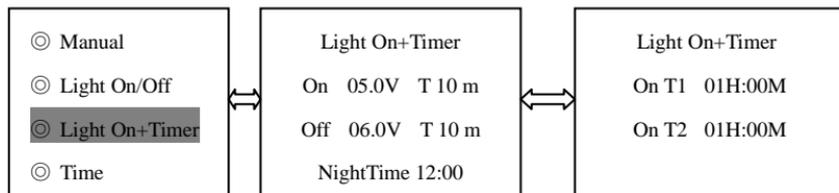
Load control mode can be set to light + time control in this interface. Parameters in the table below:
