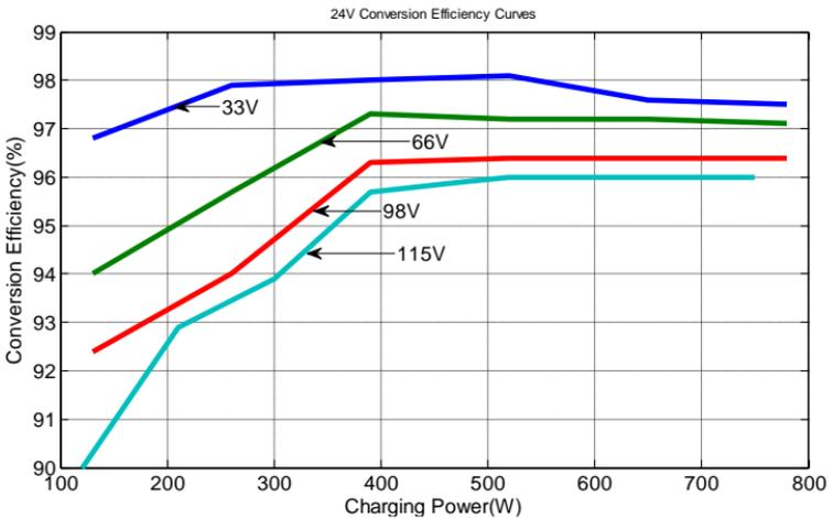
3. Solar MPPT Voltage(66V, 98V, 115V) / System Voltage(36V)
