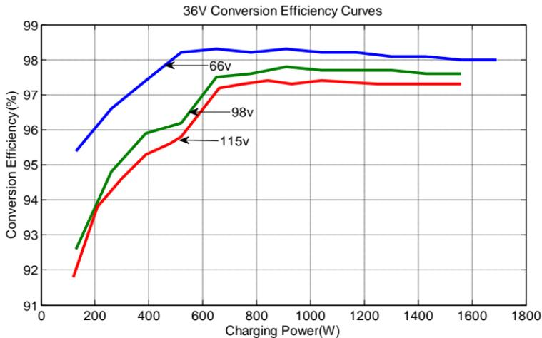
4. Solar MPPT Voltage(66V, 98V, 115V) / System Voltage(48V)
