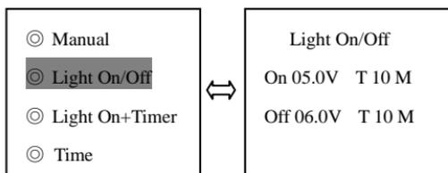
Load control mode can be set to light control in this interface. Parameters in the table below:
